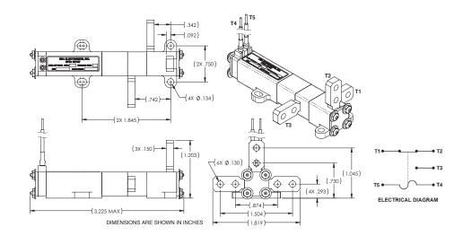
Note: Model 8023 Battery Cell Bypass Switch as an example. Other models available with alternate mounting feet, terminal configurations and optional zener diodes for autonomous operation.
