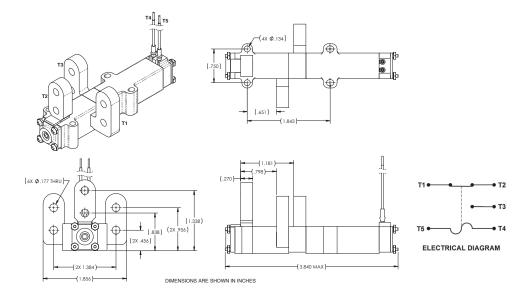
Note: Model 8036 Battery Cell Bypass Switch shown as an example. Other models available with alternate mounting feet, terminal configurations and optional zener diodes for autonomous operation.
