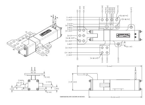
Note: Model 8043 Battery Cell Bypass Switch shown as an example. Other models available with alternate mounting feet, terminal configurations and optional zener diodes for autonomous operation.
