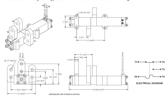
Note: Model 8030 Battery Cell Bypass Switch as an example. Other models available with alternate mounting feet, terminal configurations and optional zener diodes for autonomous operation.
