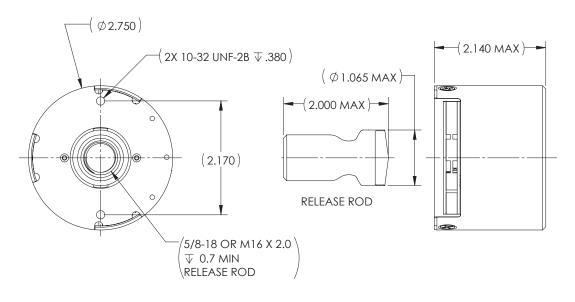
Note: Model 9106B Release Mechanism shown. Different configurations available with alternate release rods, mounting features, and connectors. Metric configurations are also available.
