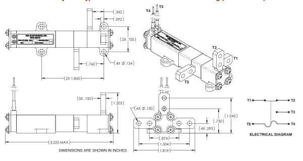
Note: Model 8020 Battery Cell Bypass Switch as an example. Other models available with alternate mounting feet, terminal configurations and optional zener diodes for autonomous operation.
